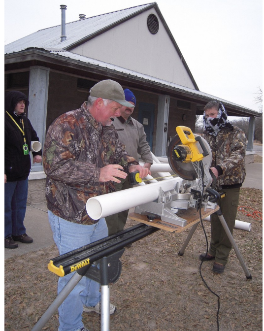
Jim Duerr and Jake Stiltz custom fit the PVC baffle to each nesting box pole.
